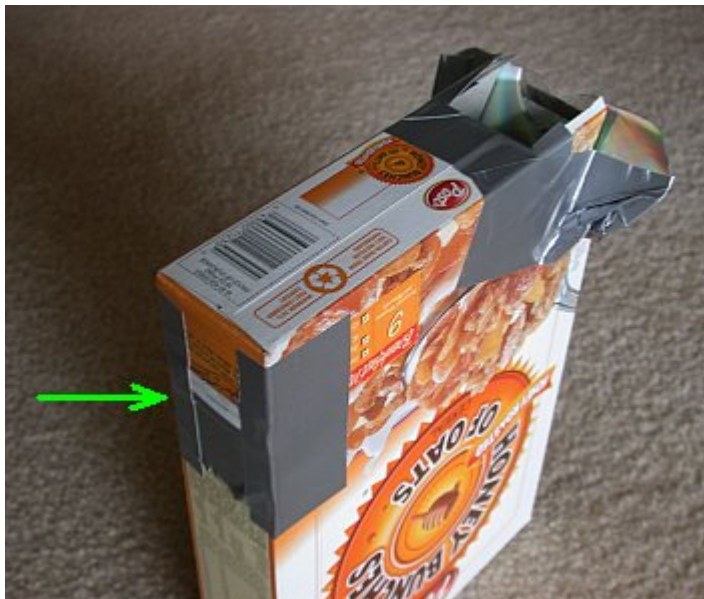
my cereal box spectroscopy (arrow: the slit)
